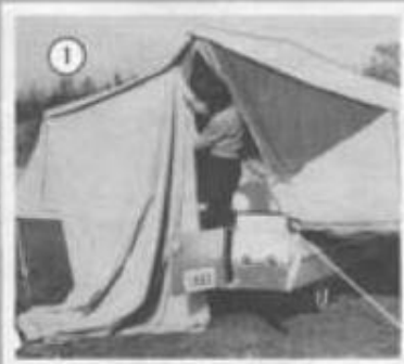
1 Tie rope from loop on peak of tent to trailer coupler - zip canopy to tent.
